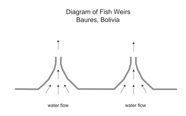
Figure 8: Diagram of a fish weirs in Baures.
