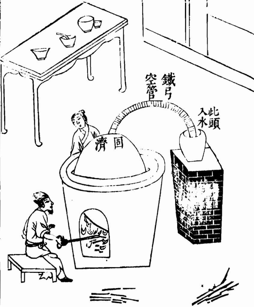
Figure 7.5. Commercial distillation of mercury, from the Technological Encyclopedia of 1637 .
